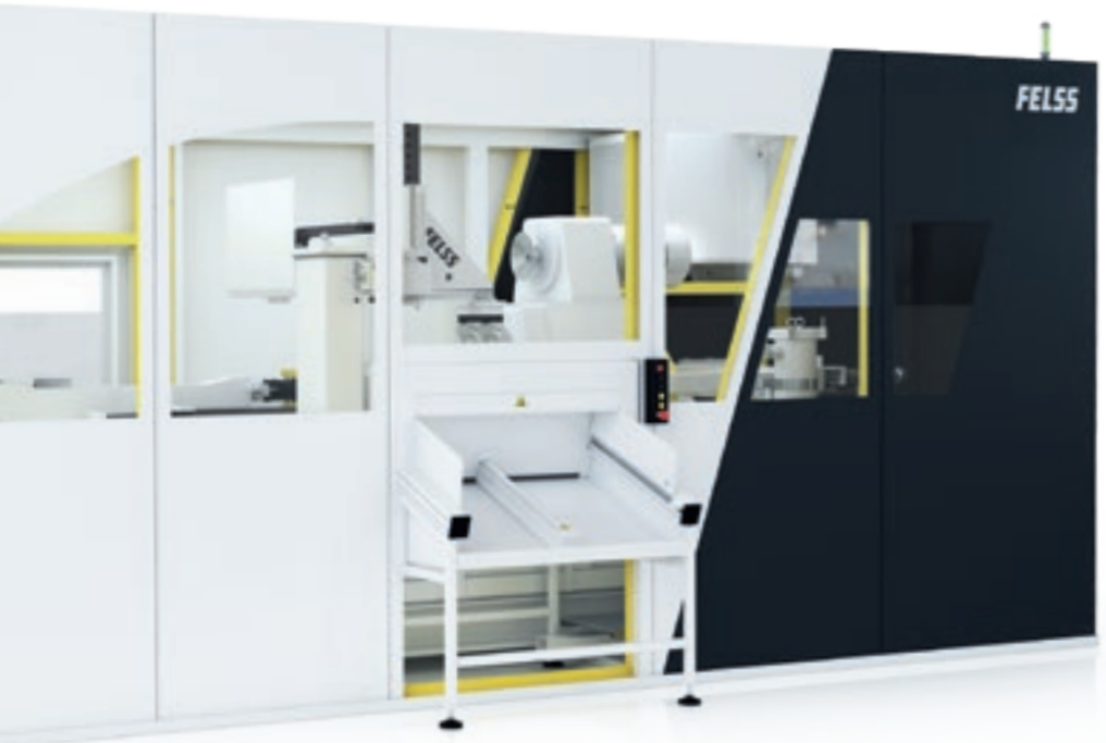
Fully automated single station swaging machines example: model HA 60-1VUEH-NC
